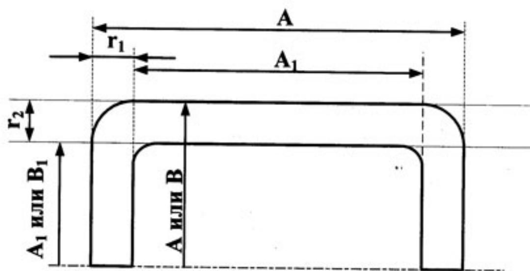
$$r_1 = \frac{A - A_1}{2}; \quad r_2 = \frac{B - B_1}{2}$$
